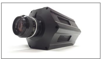
This lattice matched InGaAs camera allows for high resolution SWIR imaging 1280x1024 at high frame rates >93fps at full frame size. This small pitch array,  $12\mu m$ , combined with the high quantum efficiency of the lattice matched InGaAs arrays enables impressive imaging in the SWIR and visible band. The camera has the capability of four setpoints, 20C (no cooling), 0C (fan cooling), -40C, or -60C (water cooled) using a 3 stage TEC integrated in a vacuum package.
