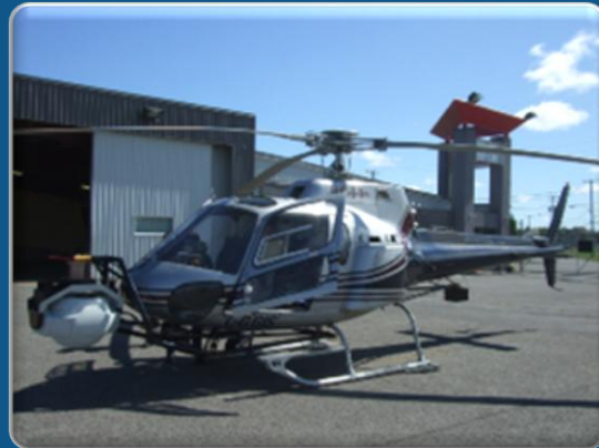
Figure 1: Telops Hyper-Cam mounted into a Gimbal on a helicopter
