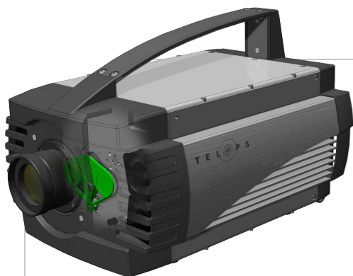
The automated 3-position filter mechanism.
